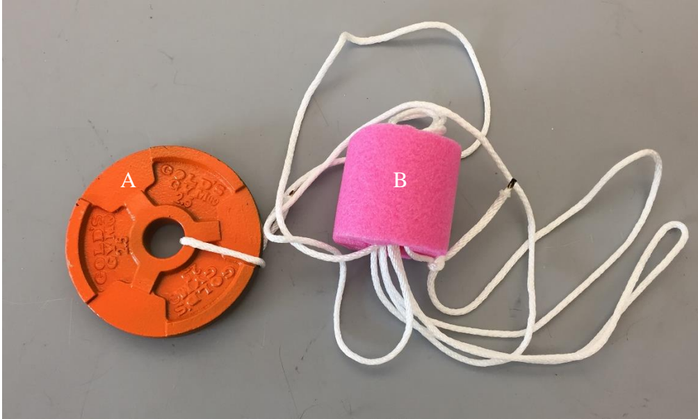
Figure 4: Control markers were placed in the survey area before the drone flights to mark locations that would be used to validate drone imagery, as they were easily spotted from all flight altitudes. The pink float aided in finding the markers from the kayak and was used for retrieval. Markers consisted of 14 cm diameter 2.5 lbs. (1.13 kg) weight (A), painted orange, and attached to a section of pool float (B) by a 5 m length of line.
